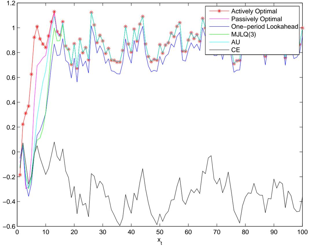
**Figure 40:** Simulated single time-series of target state  $x_t$  under different policies. Parameter values:  $\alpha = -0.05$ ,  $\gamma = 0.9$ ,  $\delta = 0.75$ ,  $\sigma_\epsilon^2 = 0.01$ ,  $\sigma_\eta^2 = 0.0001$ ,  $\omega = 1.0$ ,  $x^* = 1.0$ ,  $u^* = 0$ . Starting values:  $x_0 = 0$ ,  $\mu_0 = -0.1$ ,  $\Sigma_t = 0.04$ . True initial slope:  $\beta_1 = 0.5$ . Number of time periods:  $T = 100$ .
